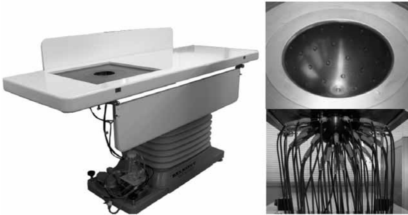
Figure 4 Mensurative bed and semispherical gantry (where 46 probes were set).
