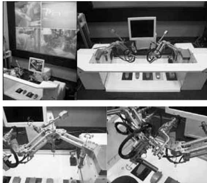
Figure 2 Master manipulators. A: Overview of the operation site. B: Master manipulators, foot switches and a display. C: Translational motion part of the master manipulator. D: Rotational motion and grasp part of the master manipulator.
