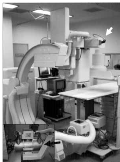
Figure 1 In-house micro-angiographic system. In-house micro-angiographic system consists of a high-voltage power X-ray source (black arrow) and a detecting system with high levels of spatial resolution and sensitivity (white arrow).
