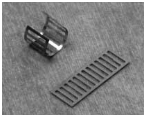
Figure 2 The stainless steel plate with the minute projections.
