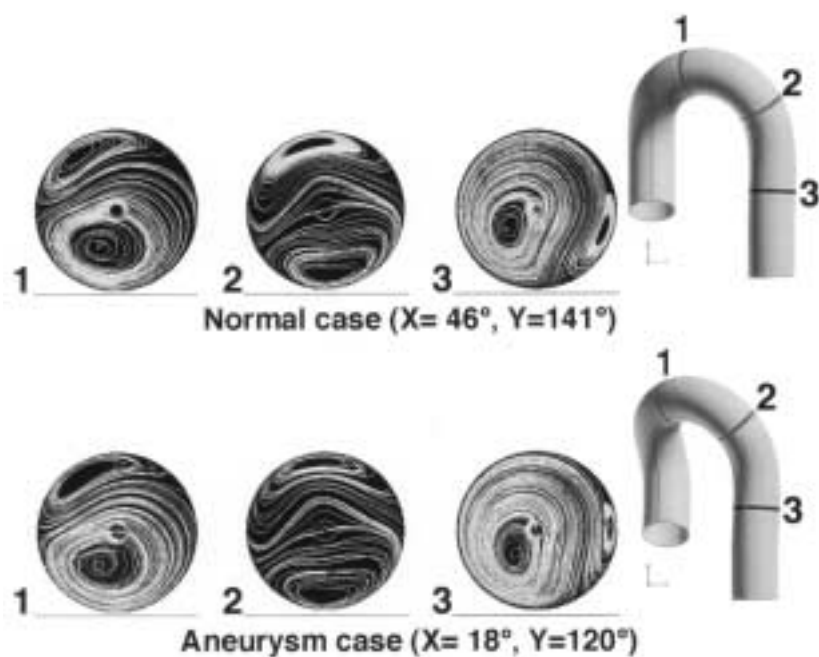
Figure 3 Secondary flow pattern at certain cross sections along the arch.
